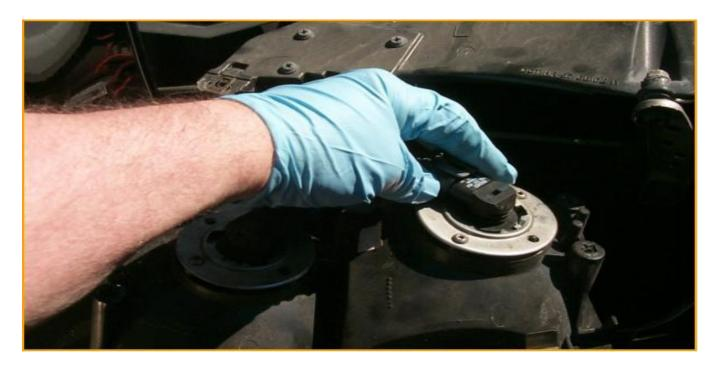
Wearing nitrile gloves is a good idea to eliminate the chance of touching the new bulb's element. Push the new bulb into the headlight assembly and twist it until it snaps in place. It will only fit one way, so you can't get it wrong
