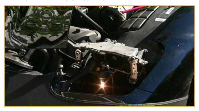
Snap the new bulb into the harness and turn the headlights on just to make sure the replacement bulb lights up as it should. If there's a problem, now's the time to find out about it rather than after you get everything buttoned back up.
