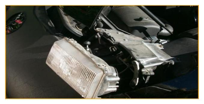
With the three retaining bolts removed, you can pull the headlight free. Here you see it out of its housing with the upper frame piece removed
