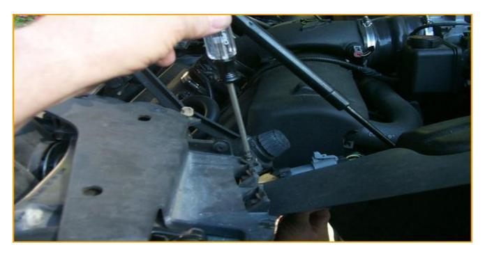
Four Torx screws are used to retain the upper headlight frame assembly, and these are removed next. When they are out, you can lift off the upper frame. Be careful not to drop any of the washers that may be used as spacers.
