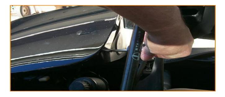
The headlight surround trim is the next item that has to be removed. It is held in place with three Phillips screws: one on the inside of the headlight and two on the outside. A stubby #2 Phillips driver comes in handy for chores like removing the inner screw, shown here
