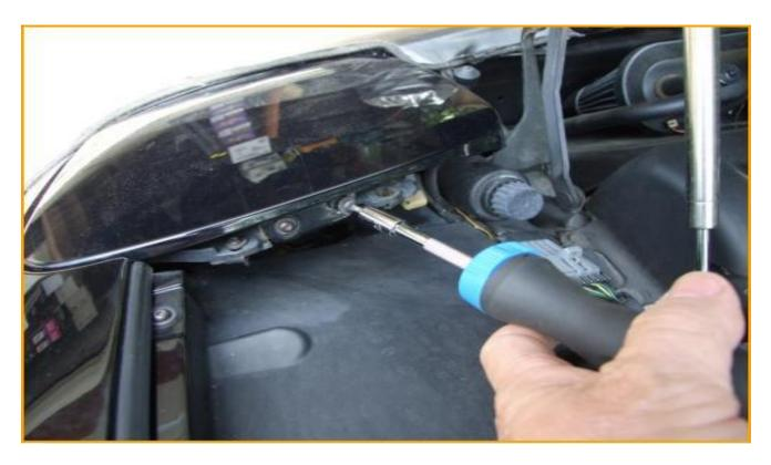
With the hood open, but with the headlights still in the down position, use the Torx driver to remove the two Torx screws that hold the rear of the headlight cover in place. When these are out, you can open the headlights so that they are in the up position.
