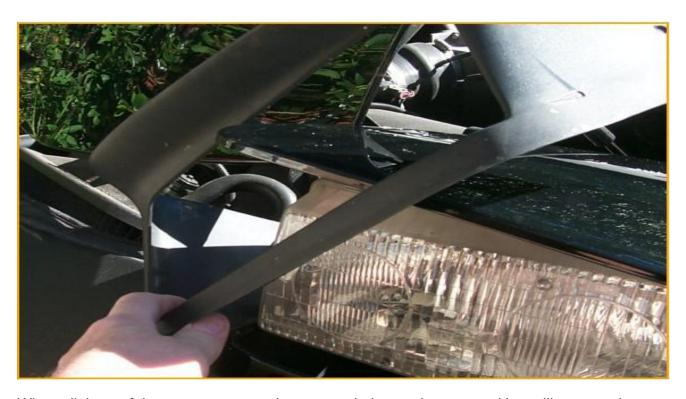
When all three of the screws are out, the surround trim can be removed by pulling up and outward on it at the same time.
