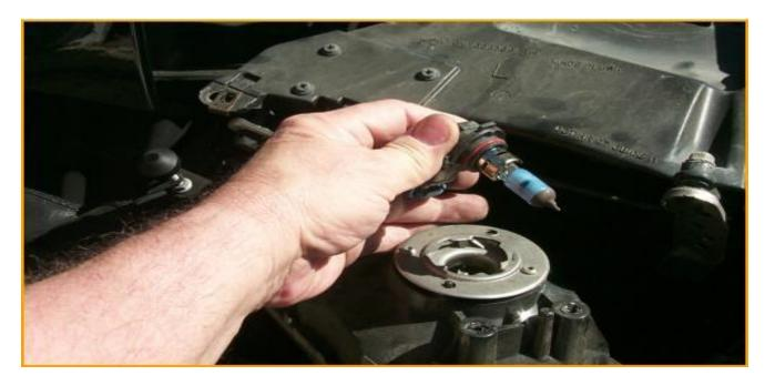
Removing the old headlight bulb is simply a twist-and-pull operation. Be careful not to touch the glass element of the new bulb, since the oils on your fingers can shorten its life considerably. The bulb, with its plug, simply unsnaps from the harness.
