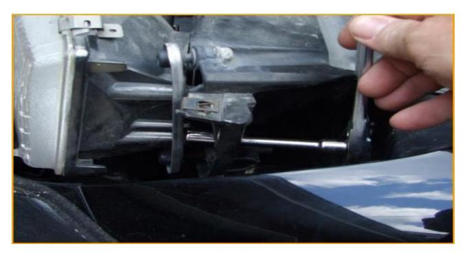
With the upper frame out of the way, accessing the three 10mm bolts that hold the headlight in place is considerably easier. Two of these bolts are on the outside, and one is on the inner side. A ¼" drive socket with extension does the trick nicely. Be careful not to drop the bolts as you're removing them, otherwise you'll need a magnetic wand for their retrieval.
