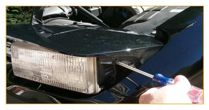
The two remaining Torx screws that are still holding the headlight cover in place, one each on the inside and outside of the headlight assembly, are removed next. The headlight cover can then be lifted off.
